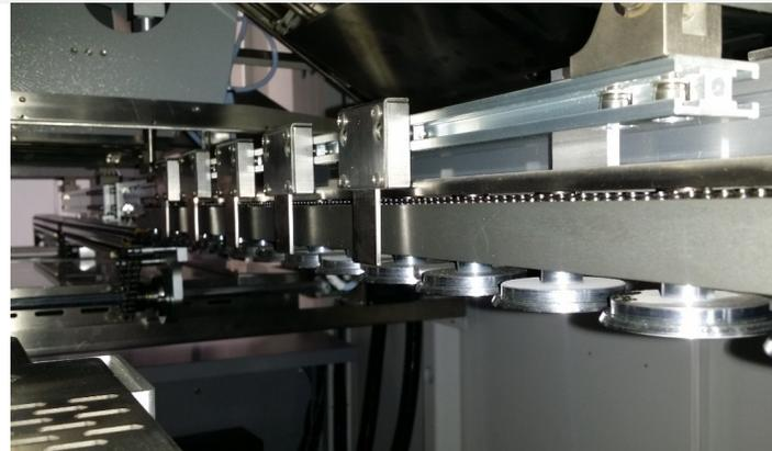
Unique heavy duty board clamping system ensures stability of PCB during soldering and fluxing.
