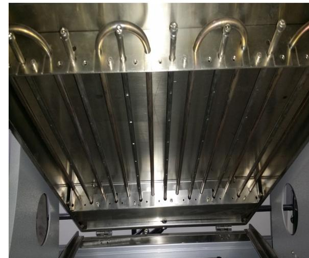
Topside convection heaters ensure the best soldering results even on the most challenging assemblies. Top heaters can be installed directly over the bottom preheat for additional preheating and/or directly over the solder pot for continuous process heat.
