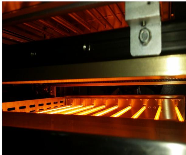
Fast reacting quartz IR preheater as standard options ensures precise preheating and flux activation before soldering.
